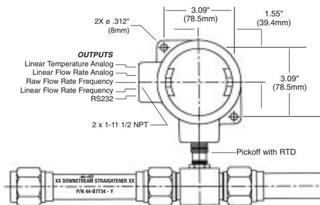
**Flowmeter & Flow Straightener with Integral RTD**
